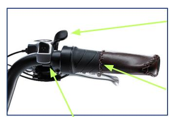
Press lever to shift gears "down" (easier to pedal, good for uphill).
