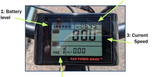
4: Pedal assist level (0-5). Press up/down arrows to change level.
