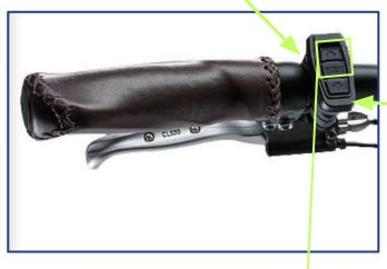
Press up/down arrow buttons to change pedal assist level.
